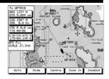
After centring the screen around the boat or cursor you can change the scale by pressing the Zoom In or ZoomOut keys and the TRACKER950 will retain the scale selected. This is useful. For example, you can:
